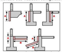
A or A+ B must equal two feet in Zone 5 or four feet in Zone 6
